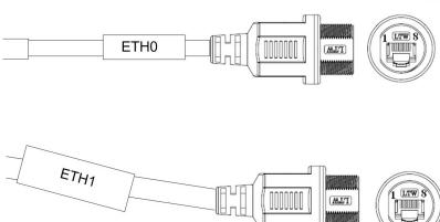
PIN1: DA+ POE V+ PIN2: DA- POE V+ PIN3: DB+ POE V-PIN4: DC+ POE V+ PIN5: DC-POE V+ PIN6: DB-POE V-PIN7: DD+ POE V-PIN8: DD-POE V-
